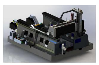
High performance Gantry Milling Machine. Its configuration and design allow the machining of large parts and parts of varied morphology, combining highly effective chip removal capabilities with an excellent finish quality.
